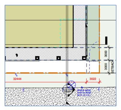
• Swept paths have not been provided for all access ramps and the basement design requires a number of hook turns, some of which appear problematic/impossible such as the vehicle movement required for vehicles entering 'Basement 2' (left hook turn required at bottom of ramp).
