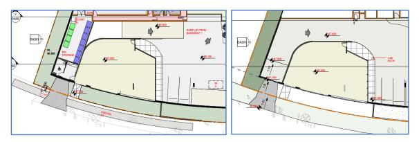
• The lift locations for *Building C* do not align, with the location of the lift shaft in the basement out of alignment with the lift location above ground (as indicated in the below images).
