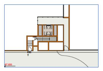
• The driveway entry to the mezzanine car park level off Digitaria Drive at the eastern end of the site (below *Building C*) indicates the entry/exit arrows on the wrong side of the road/driveway. There is also vehicle conflict with vehicles that have entered this parking level from the western driveway.
